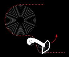
STEP 3: With the chain now cut to length it is important to test the clearance of the OSPW System when rear derailleur is set in the biggest chain ring and the largest cog on the cassette. Just as the arrow indicates the cage should be able to rotate counter clockwise. It is important that there is some clearance between the upper pulley wheel of the OSPW System and the largest cog on the cassette. If you find the clearance is not enough, adjust the B-tension accordingly.
