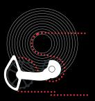
STEP 1: Place the chain on the small chain ring and the smallest cog on the cassette. To find the correct chain length, pull the two chain ends together, just as you would when needing to cut a chain to length. The lower part of the cage should start to move downwards, away from the cassette, as referenced in the second image.
