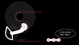
STEP 2: When tension is applied on the chain and the OSPW System appears to be aligned as the diagram above, the chain needs to be cut (1 link shorter than step 1) and connected by the required amount of links in order to achieve sufficient tension in this gear combination (always the small cog on the cassette).
